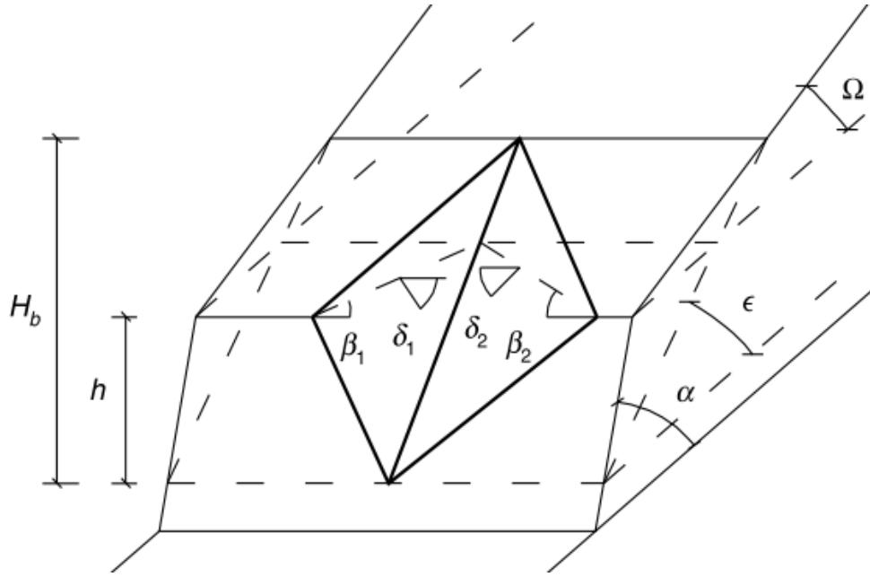
$$FS = \left( a_1 - \frac{b_1 G_w}{S_\gamma} \right) * \tan\phi_1 + \left( a_2 - \frac{b_2 G_w}{S_\gamma} \right) * \tan\phi_2 + 3b_1 \frac{c_1}{\gamma h} + 3b_2 \frac{c_2}{\gamma h}$$
