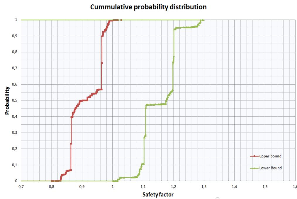
Bounded cumulative probability distribution of the factor of safety, calculated by random sets with assigning 90% of the probability to one interval
